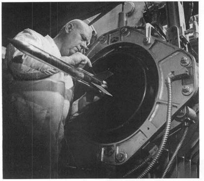
MODEL ROCKET underwent stability tests at Mach 7.5 in Sandia's new hypersonic wind tunnel last month marking the beginning of regular testing in the new facility. Cecil Tolbert adjusts balance mount.
